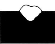
This causes excessive penetration with spatter and deep pointed crater. It may also cause holes to be burned in the workpiece.
