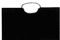
This causes irregular masses of weld to be deposited, with slag contamination on an uneven surface.
