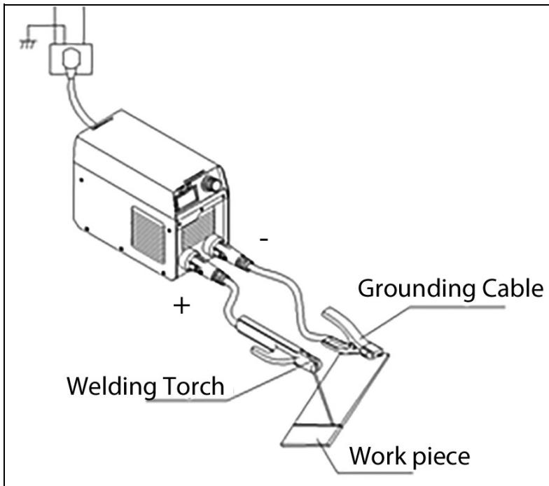
4. Select the appropriate welding rod and insert it into the welding rod holder.
