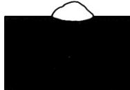
This causes poor penetration and causes the electrode to stick to the workpiece too readily. Also results in a very irregular and high weld deposit. Slag is very hard to remove.
